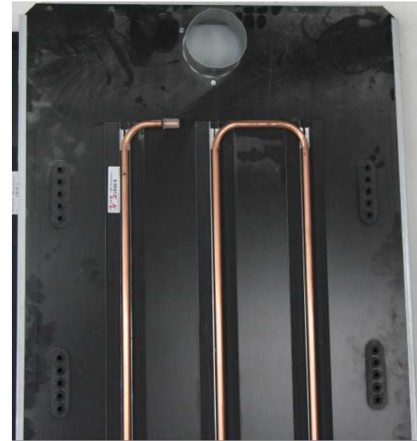
The surface of the hybrid Ducts are activated with Copper Tube Meander
